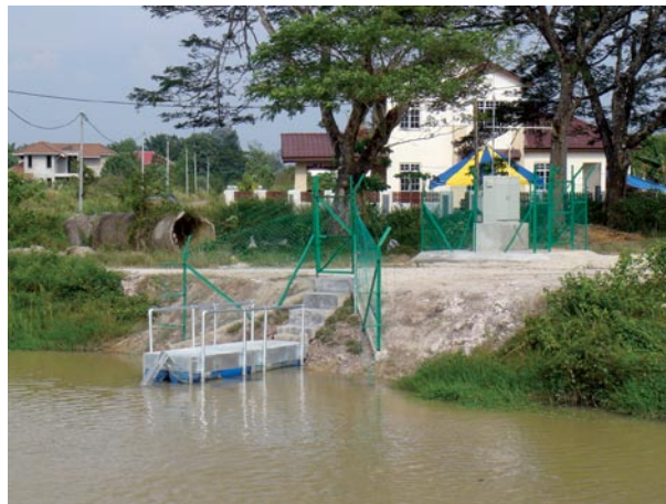
On contract with the Malaysian government, ASMA uses 15 unattended continuous monitoring stations to safeguard drinking water supplies and collect extensive data on water quality.
